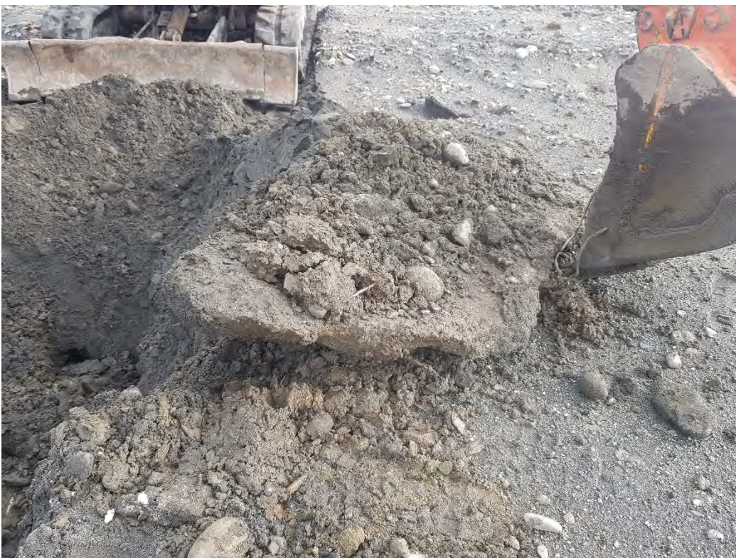
Photo 4. Concrete block encountered at Test Pit SP2 at 0.3 m bgl.
