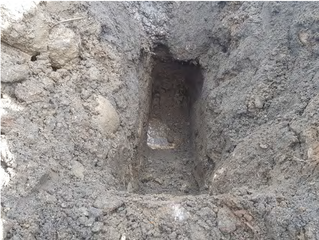
Photo 3. Test Pit SP2 showing organic matter and groundwater at depth (1.3 – 1.4 m bgl).
