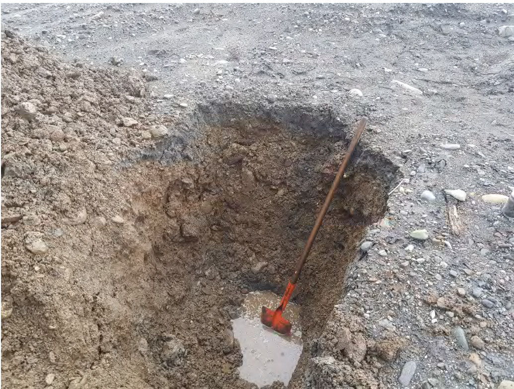
Photo 10. Close up of Test Pit SP5. Trace asphalt observed near surface.
