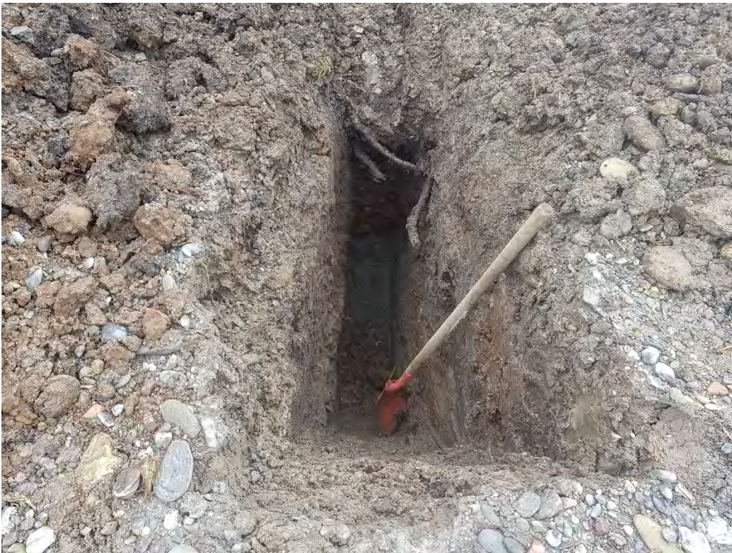
Photo 8. Close up of Test Pit SP4. No demolition waste material was observed.
