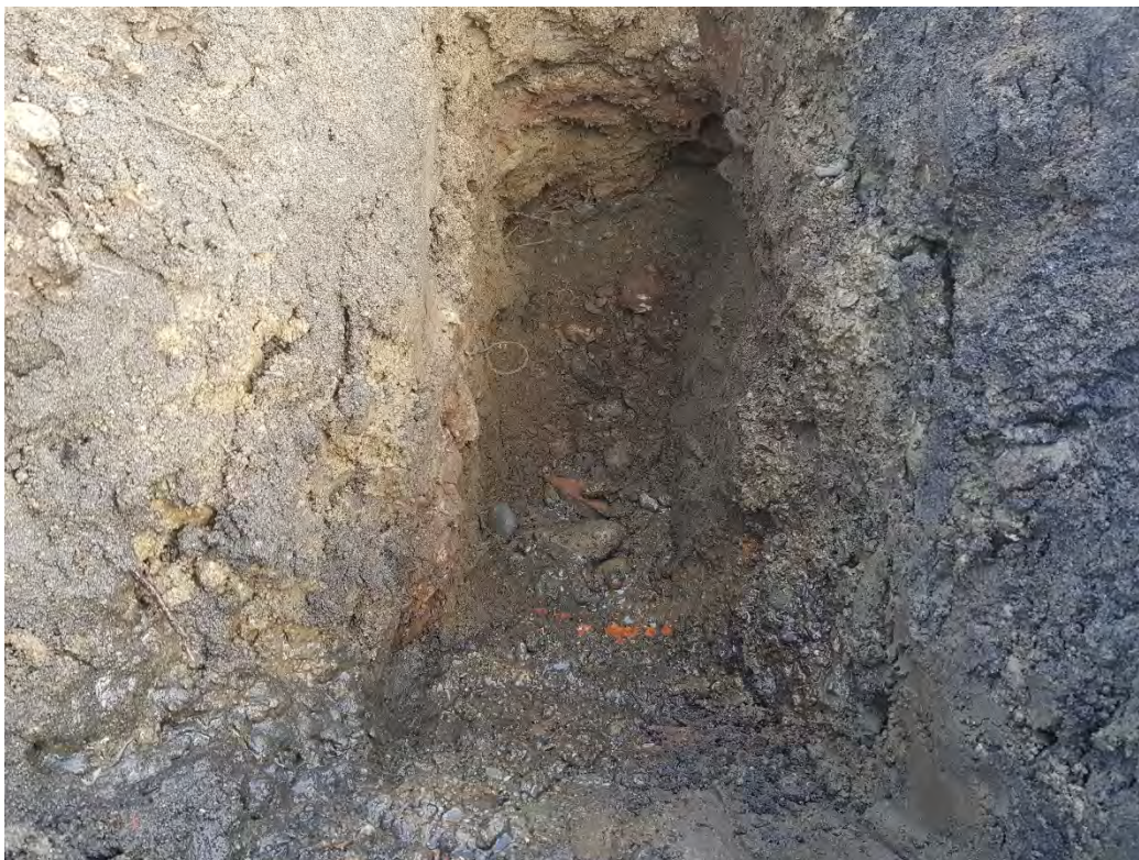
Photo 2. Test Pit SP1 showing demolition waste (bricks, concrete, wire) at depth (1.3 – 1.4 m bgl).
