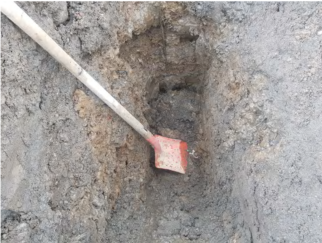
Photo 6. Close up of Test Pit SP3. Trace asphalt observed at 0.4 m bgl.
