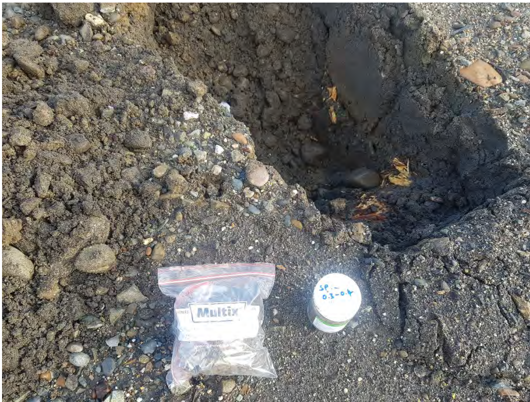
Photo 1. Test Pit SP1 showing wood debris in sandy silt matrix.
