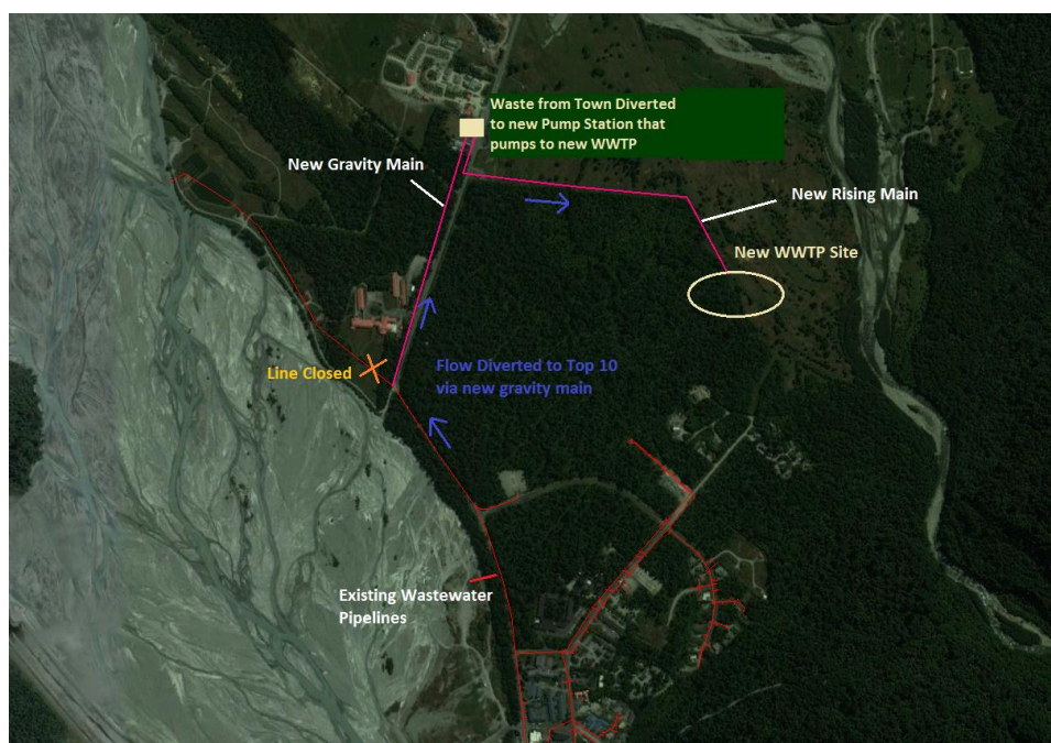
Figure 19: New Wastewater Mains and Pump Stations for Sites 1, 2 and 3
