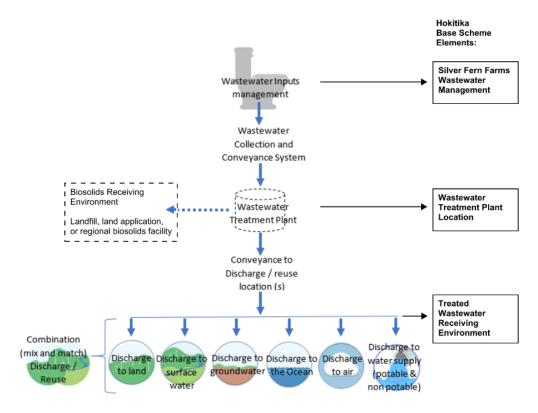
Figure 1: Hokitika Wastewater Base Scheme Elements
