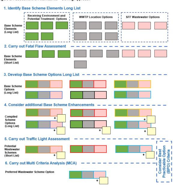
Figure 3: Options Assessment Process - Schematic Layout
